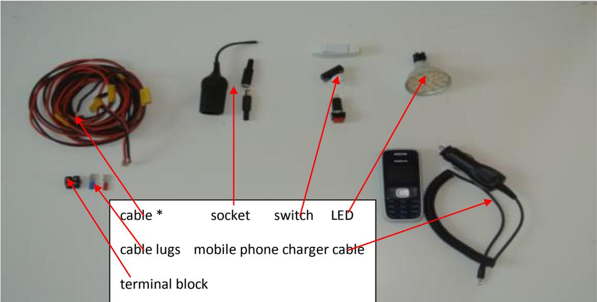
\* The cable connecting the solar module with the solar controller should be 2.5 mm thick and 5 m long; the cable to the light source should be 1 to 1.5 mm thick and 10 m long since the cables in West Africa are usually not made of copper but of an iron alloy. The stronger the cable, the better!
