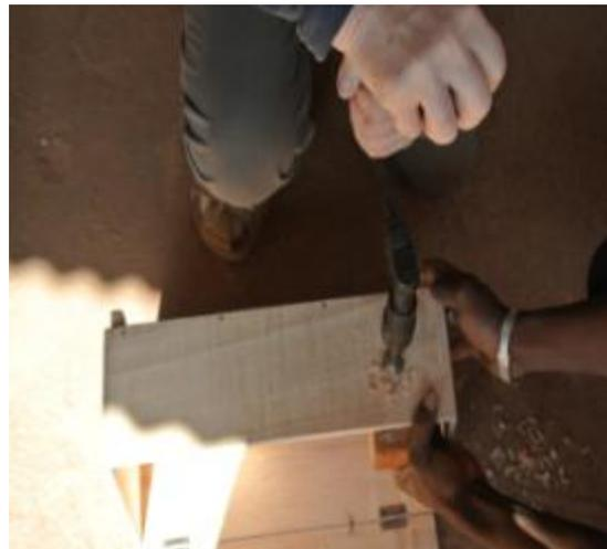
All sorts of materials are suitable for making a casing, including larger calabashes with a wooden board as bottom. Number and size of the holes depend on the parts to be fitted. A small drawing before drilling will be helpful. The drawing will show where the charge controller, the connectors and the switches are to be fitted.
