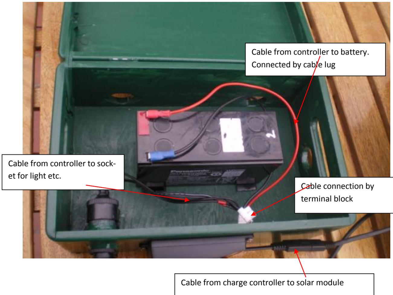
This is the simple finished solar home system for lighting and charging of mobile phones
