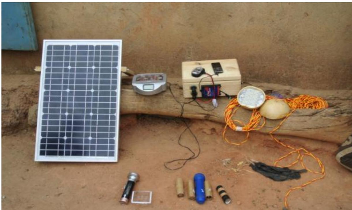
This is a small solar home system (SHS) of 20 watts for lighting, cell phone charging and charging rechargeable batteries for flashlights.
