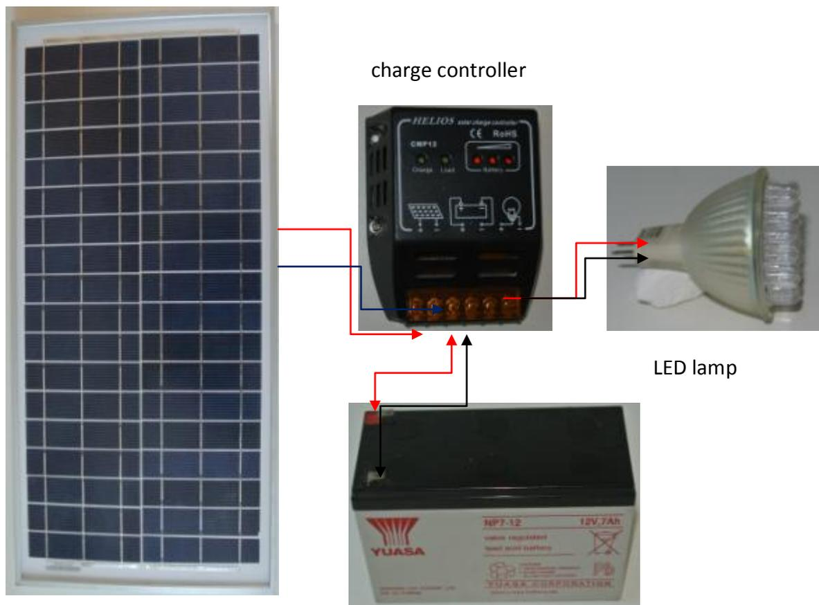
The light falls on the solar panel and stimulates the production of electricity. Via the connecting cable (red for plus, black for minus), the current flows into the charge controller and from there to the battery. When a lamp is connected, the current flows back from the battery through the charge controller into the LED lamp, which is then lit up.
